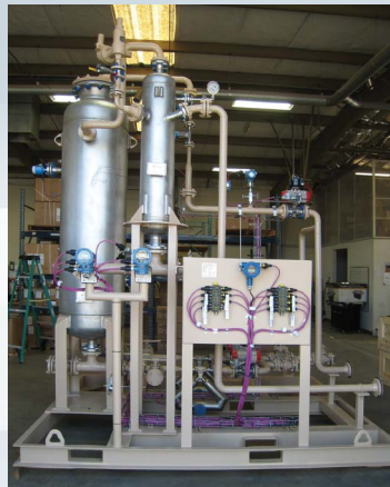
3-phase JR in Duplex Stainless Steel
